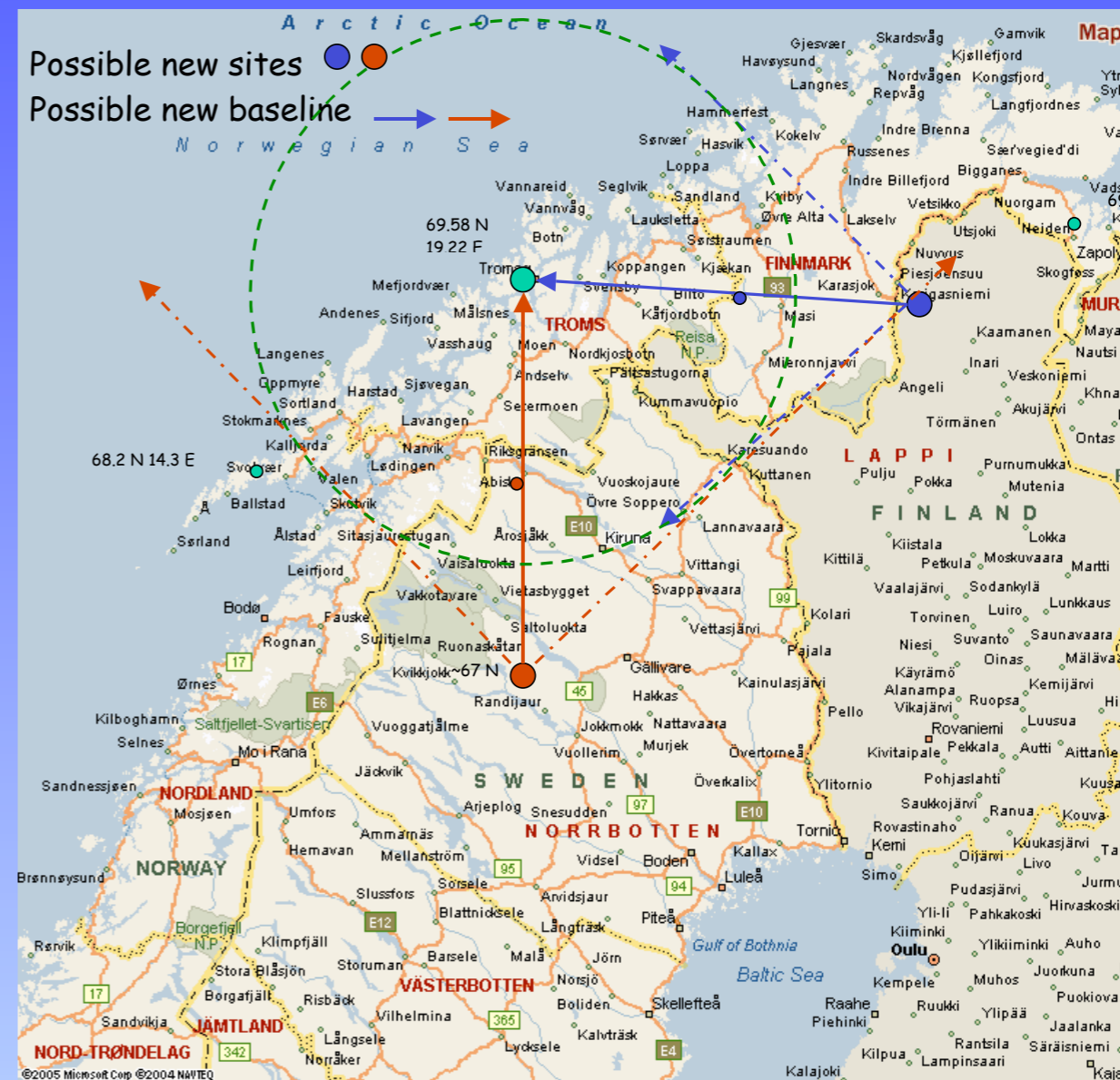
The figure shows one possible layout of the EISCAT 3D system. In this configuration, the central core (denoted by a green filled circle) is assumed to be located near the present Norwegian EISCAT site at Ramfjordmoen. The dashed circle with a radius of approximately 250 km indicates the approximate extent of the field-of-view of the central core at 300 km altitude. Phased-array receiving sites located near Porjus (Sweden) and Kaamanen (Finland) provide 3D coverage over the (250-800) km height range, while two additional receiving sites near Abisko (Sweden) and Masi (Norway) cover the (70-300) km height range.
