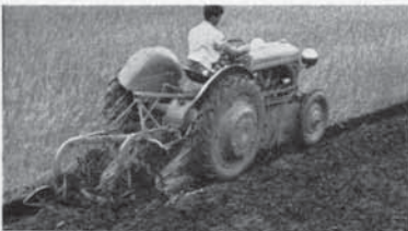
The Ford tractor and hydraulically controlled, wheelless plow are designed and built as a unit. The basic idea of this development is to permit economical and profitable mechanized operation of small as well as large farms.
